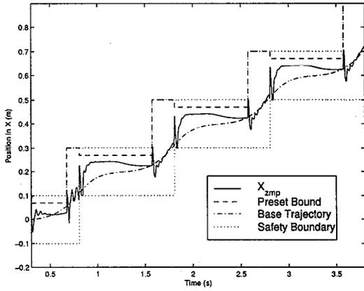
Figure 4: ZMP trajectory without disturbance
