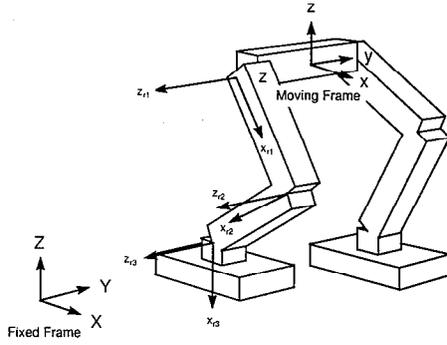
Figure 1: Coordinate frames of the biped robot
