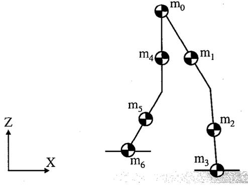
Figure 2: Model of the biped robot as a system of particles
