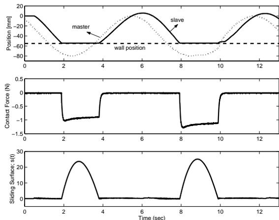
Figure 8: Position, external force, and sliding surface with the modified SMC (RTT $\approx$ 1.5 s).
