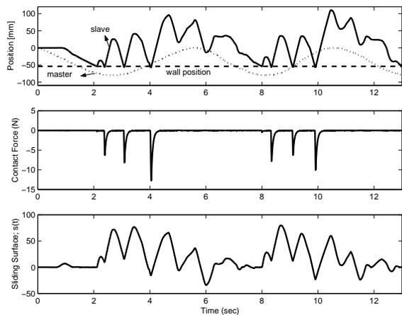
Figure 7: Position, external force, and sliding surface with the regular SMC (RTT $\approx$ 1.5 s).
