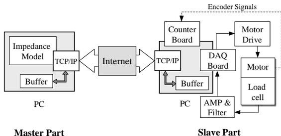
Figure 5: A detailed description of the master/slave system.
