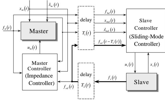
Figure 2: The overall system block diagram.
