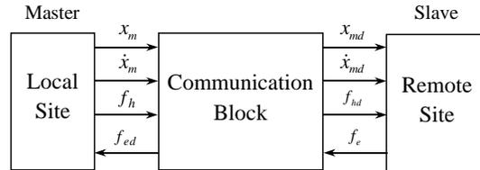
Figure 1: A block diagram of bilateral teleoperation.
