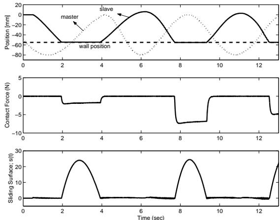
Figure 9: Position, external force, and sliding surface with the modified SMC (RTT $\approx$ 4.0 s).
