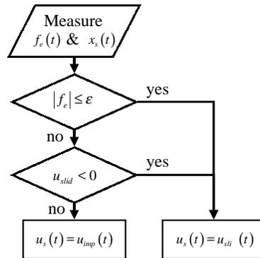
Figure 6: Flow chart for the control input selection.
