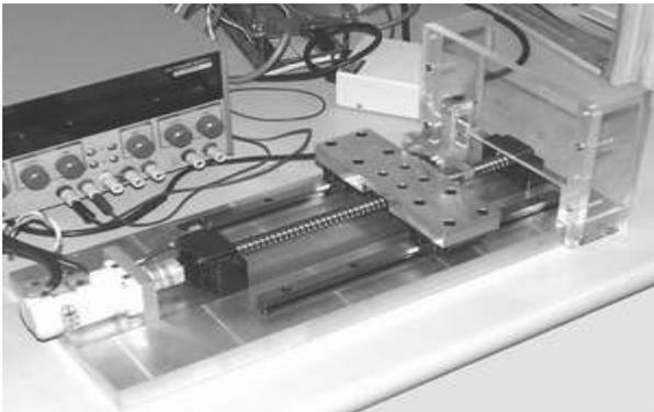
Figure 4: The slave system used in this experiment.
