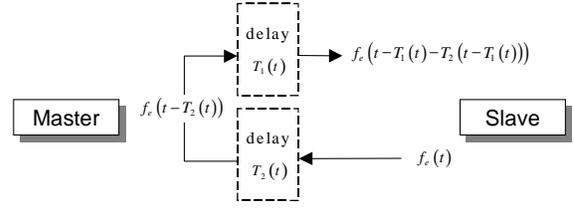
Figure 3: Delayed force signals for the modified sliding-mode controller.
