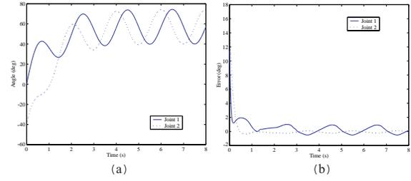
Figure 1: (a) Desired trajectories of joints (b) Position errors of joints
