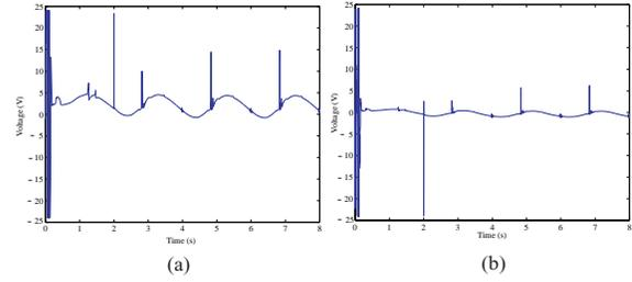
Figure 2: (a) Voltage of actuator of joint 1 (b) Voltage of actuator of joint 2
