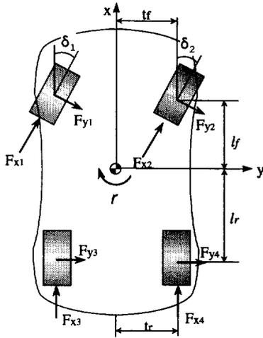
Fig. 1. A front-wheel-driven vehicle model and its related forces.
