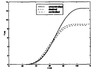
Fig. 7. Vehicle trajectory during a lane change on a slippery road.
