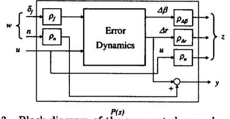
Fig. 3. Block diagram of the augmented error dynamics.
