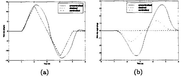
Fig. 6. (a) Yaw rate and (b) side slip angle during a lane change on a slippery road.
